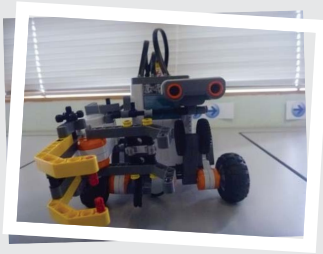
This robot equipped an arm for catching object
