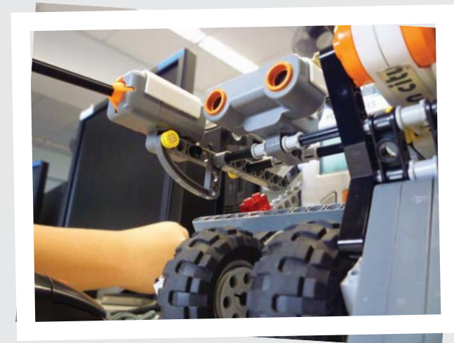
This robot can detect the distance between robot and obstacle
